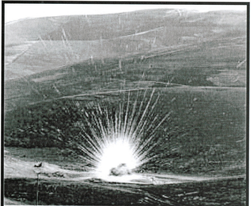
Hydrodynamic (bomb core) test on a firing table at Site 300. The "streaking" effect is from shards of pyrophoric metal, such as Uranium-238, hurtling through the air. U-238 is one of the contaminants of concern in the Site 300 Superfund cleanup.
